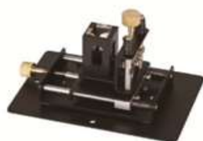
Adjustable XY micro cell holder
