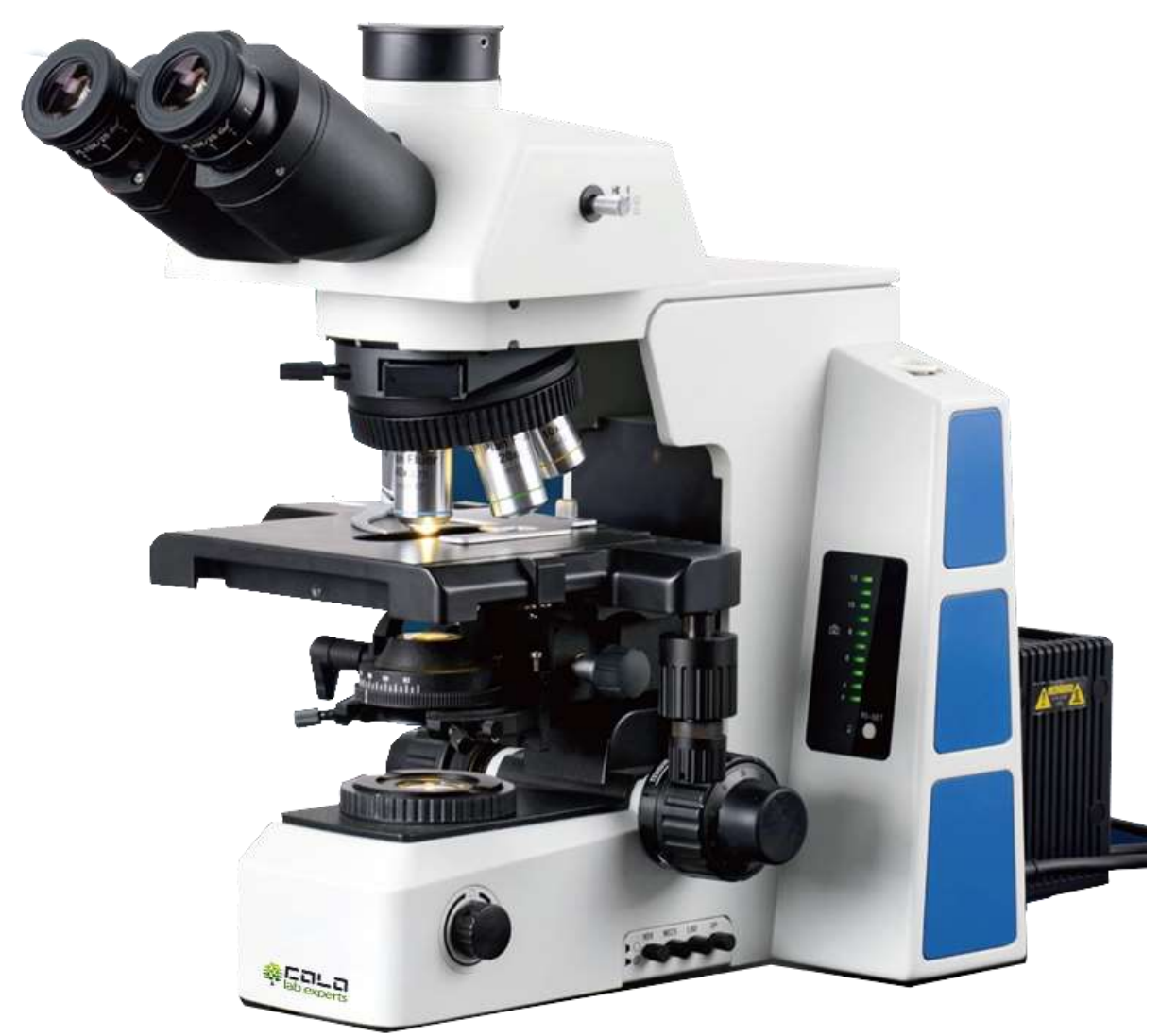
Research Scientific Laboratory Microscope, Semi-APO, Upgrade +DF+PL+PH+FL+DIC
