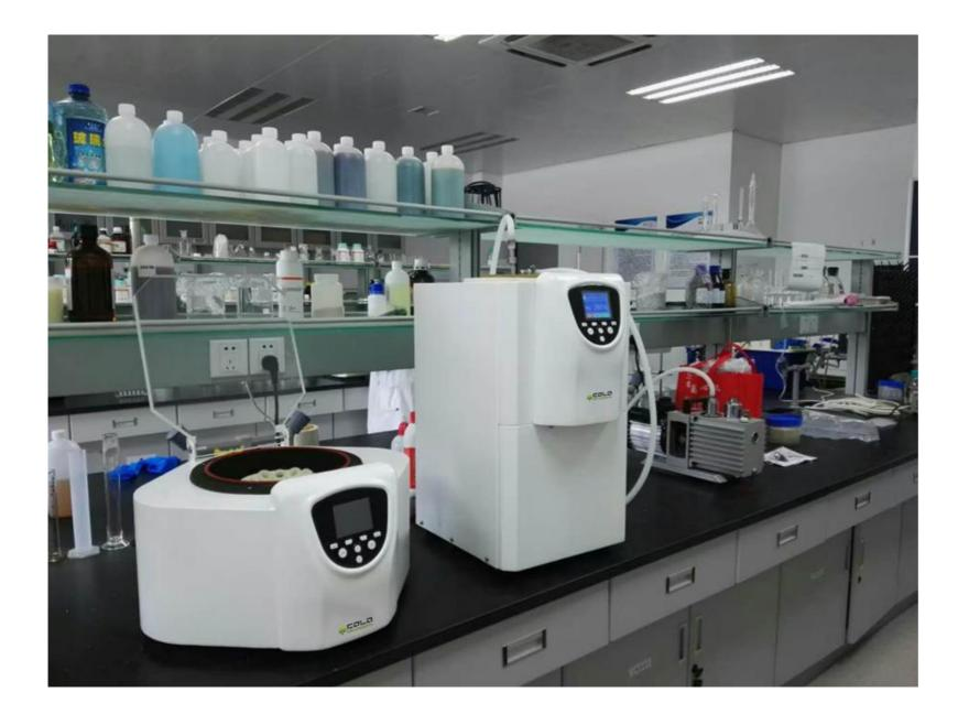
Can quickly evaporate or remove the water and organic solvents from the sample. The processed sample can be conveniently used for the purpose testing and research, widely used for various qualitative and quantitative analyses. Chemical analysis biological analysis, immune screening, food safety, residue analysis ....
